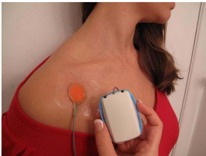
Figure 2. The wearable low-intensity therapeutic ultrasound (LITUS) device (worn by a modeled) shown as used as in this shoulder pain study. Patients wore the device for approximately 3.5 hrs on a daily basis.
